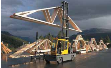
■ A Baumann sideloader moves a roof truss to a collection point.
